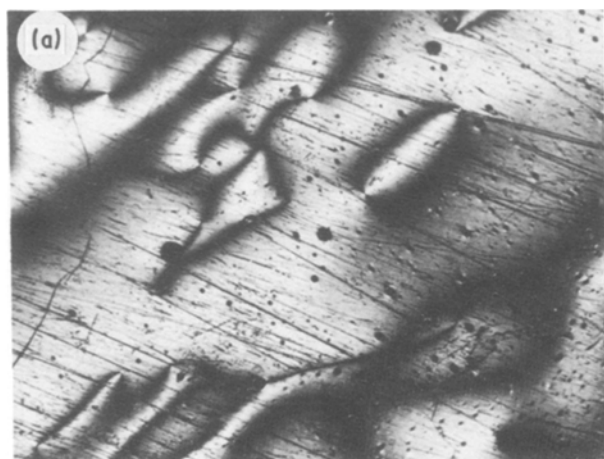
Figure 1 Optical photomicrographs of mesophase pitch and its blends with 5 and 10% PPO. (a) Mesophase pitch, (b) 5% PPO, (c) 10% PPO.
